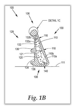
Figure 1B depicts a cross sectional side view of hollow iron golf club head 100. Ex. 1004, 3:49:50. The depicted golf club head includes striking face 110, back wall 132, and cavity 120 filled with filler material 121. *Id.* at 4:1–17. Wahl discloses that the filler material may be a "viscoelastic elastomer" or "styrene/isoprene block copolymer." *Id.* at 4:51–58.
