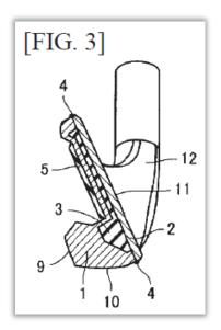
Figure 3 is a cross-sectional view of an iron golf club head. Id. ¶ 162. The depicted golf club head includes body portion 1, face part 2, and hollow portion 3, and back portion 9. Id. Mizuno discloses that hollow portion 3 is filled with an "elastic body" formed from "polyurethane resin." Id. ¶ 109.
