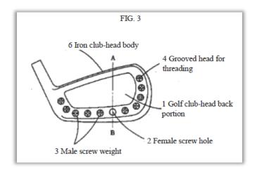
Figure 3 depicts a rear elevation of an iron golf club head. Ex.  $1006 \, \P \, 8$ . Female screw holes 2 and male screw weights 3 are located along the periphery of the rear side of the depicted golf club head. *See Id.*, Fig. 2.
