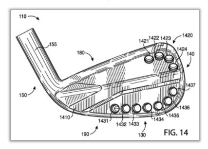
Figure 14 depicts threaded weight ports 1421–24 and 1431–37, located in the back portion 170 of body portion 110. *Id.* at 2:1–2, 5:48–57.
