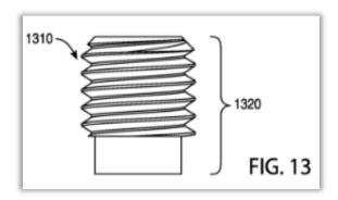
Figure 13 depicts cylindrical weight portion 130 with threads 1310 that may secure the weight portion in a weight port located in back portion 170 of the disclosed golf club head. Ex. 1001, 1:66–67, 4:25–37, 4:54–58.
